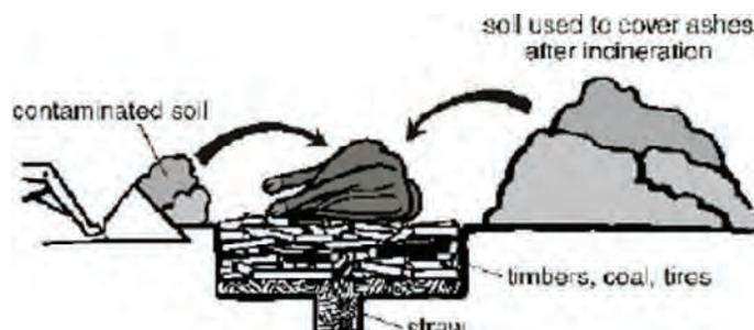
Figure C. Cross section of pit ready for burning.
